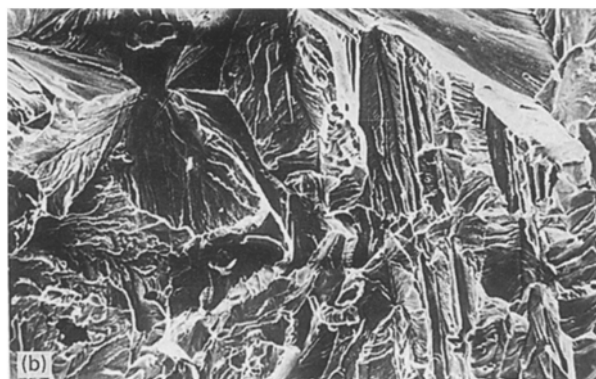
Figure 4 SEM photomicrographs of fractured tensile samples: (a) SB-WA, (b) SB- \mu A, and (c) S- \mu A.
